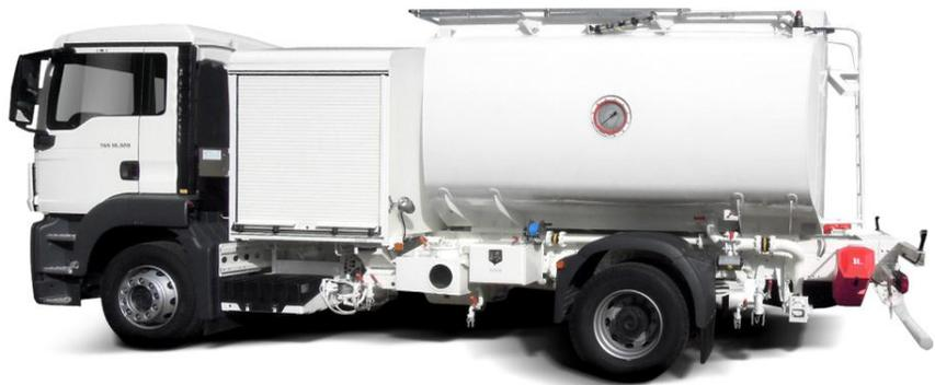
A 10,000L rigid refueller mounted on a 4x2 chassis. The refueller is equipped with 1 x underwing and 1 x overwing hose, single meter and filter water separator or an optional filter monitor. Options include a weatherproof cabinet. The refueller conforms to latest European Standards EN12312-5 and JIG1 Issue 11 requirements.
