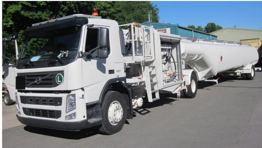
A semi-articulated refueller incorporating a 4x2 chassis and single trailer axle configuration for optimal manoeuvres on the airport ramp. The elevating platform and refuelling unit are mounted on the chassis unit immediately behind the cab, with the semi-trailer tank attached by means of a liquid 5<sup>th</sup> wheel. The refueller is designed and constructed in accordance with the latest European Standards BS EN 12312-5 and JIG 1 Issue 11 requirements where applicable.
