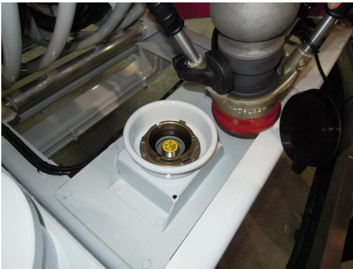
Intrinsically Safe hose reel HEPC nozzle stowage - electrical interlock.
