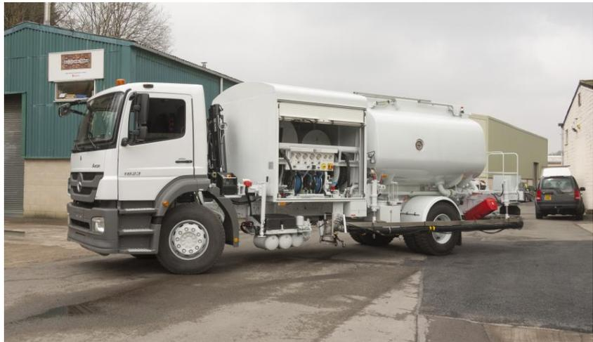
10,000L hydrant pit cleaner suitable to perform the following operations: routine flushing of hydrant pit valves, routine sampling from hydrant low point drains and purging high point vents, cleaning of hydrant pits with air, water and removal of dirt and water with vacuum suction.
